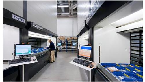
Tornado Lift machine offers safe and secure storage for storing and handling your small items in your warehouse or shop. The intelligent engine of the system attempts to place active trays close to the retrieval point. This makes the TornadoLift machine especially useful for seasonal products. Tornado has password-protected access levels for added security.
