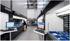
Tornado Lift machine offers safe and secure storage for storing and habdling your small items in your warehouse or shop. The intelligent engine of the system attempts to place active trays close to the retrieval point. This makes the TornadoLift machine especially useful for seasonal products. Tornado has password-protected access levels for added security.
